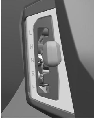
The transmission gear selector is located on the left side of the vehicle. The transmission selector lever has five positions: low gear; high gear; neutral; reverse; park.
