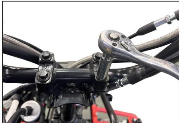
**NOTE:** Tighten bolts so there is an equal gap at the front and rear of the handlebar block. Improper gap will result in improper fit of upper pod.
